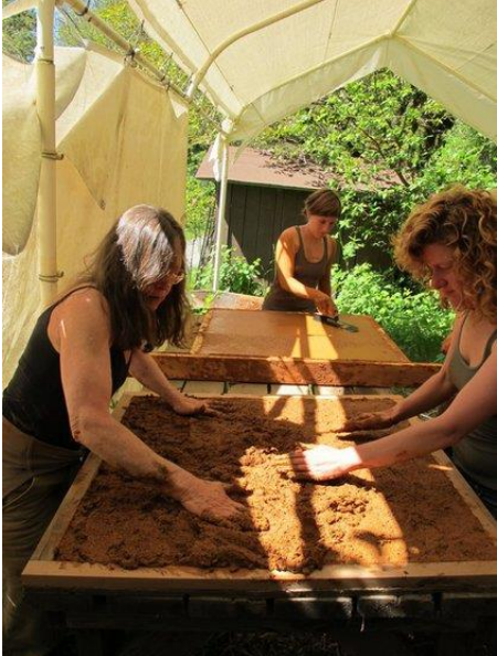
Making earthen floor test panels during Natural Building Course
